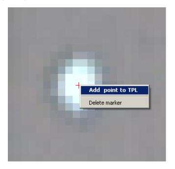
5. For every image set the correspondences between the TPL (IMAGE) tiepoints and the TPL (CALIB) tiepoints. This is done by simultaneously displaying both tiepoint lists as shown below. Establishing a link defining the correspondence is done with drag and drop. Left-click an item's name in the TPL (CALIB), drag it over the corresponding name in the TPL (IMAGE) and drop it. You see the link in the link column.
