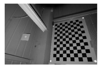
For calibration the flat check pattern is captured by the camera to be calibrated several times. The whole image area should be covered, and in each image the complete pattern has to be visible. The inner check pattern corners are automatically detected by the calibration software and are automatically linked to the 3D coordinates of the flat check pattern corners (z is always 0).
